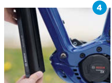
Removing the battery from the frame
