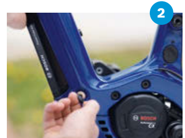
When the battery is unlocked using a key (depending on the manufacturer), it automatically drops into the restraint support
